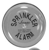
The Series 760 FireLock Water Motor Alarm is a mechanical, water-powered device signaling the flow of water in an automatic sprinkler system. The unit is usually installed on a wall with the motor inside the building and the gong outside for maximum audibility. A 100 mesh strainer with  $^{3}/_{4}$ " NPT threaded end connection is provided for compliance with NFPA 13 requirements.
