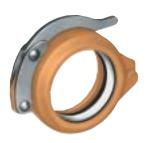
Style 78 Snap-Joint couplings are designed for quick disconnect service. Mated housings are hinged with an attached locking handle for assembly. Housings through 4" (100 mm) size have a smooth outer
