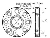
**Note:** Gray area of mating face must be free from gouges, undulations or deformities of any type for effective sealing.
