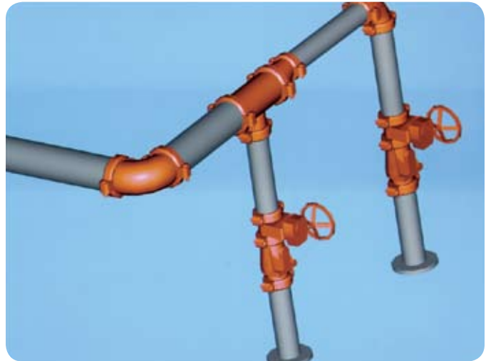
Vic-Blocks – designed specifically for AutoCAD users, Vic-Blocks 3D is a dimensionally accurate, three-dimensional block library that was developed to assist with Victaulic piping system layouts. It includes block symbols representing the main product line, drawn at full size.
